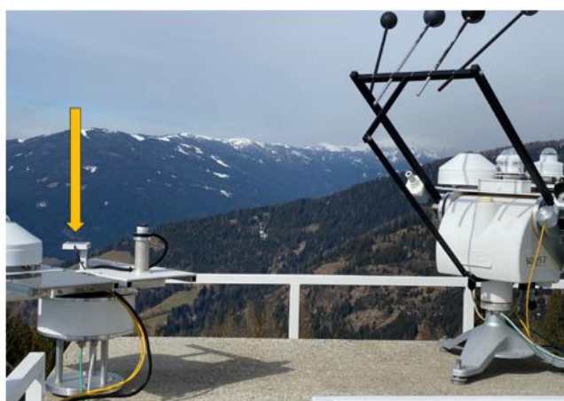
Fig1.: The picture shows a ARAD Station with the pyranometer on the right and the flat white Lightmeter Mark2.3L on the left (indicated by the yellow arrow) on the roof of the Kanzelhöhe Observatory. The picture was taken on March 12, 2023.
