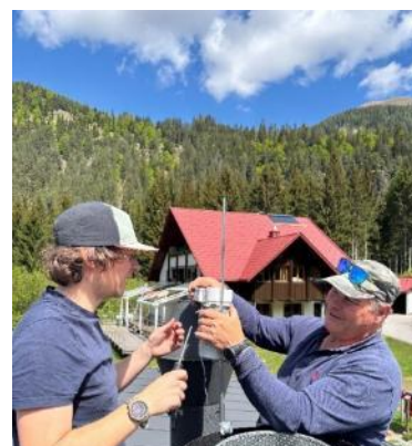
Figure 1 - Installation of the SQM and TESS-W sensors at the Weißensee Lake. Photo by Sabrina Muscolino.
