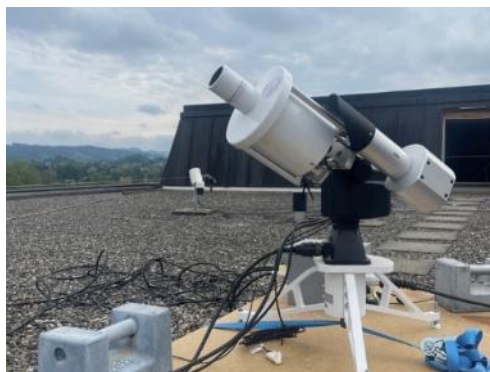
Fig. 1: multi-angle spectroradiometer on METAS roof pointing toward Bern city.
